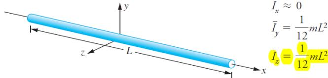
$$\begin{aligned} \bar{I}_x &\approx 0 \\ \bar{I}_y &= \frac{1}{12}mL^2 \\ \bar{I}_z &= \frac{1}{12}mL^2 \end{aligned}$$
